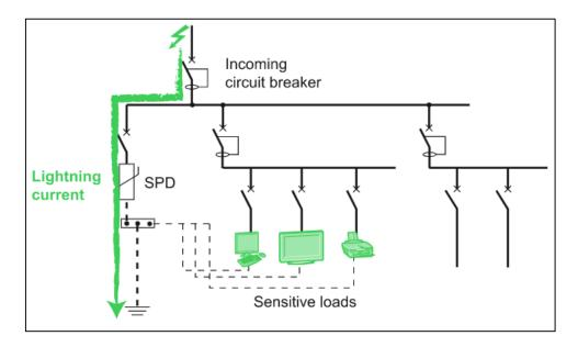
SPD connected in parallel has a high impedance. Once the transient overvoltage appears in the system, the impedance of the device decreases so surge current is driven through the SPD, bypassing the sensitive equipment.
