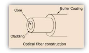
The core and cladding are usually fused silica glass covered by a plastic coating, called the buffer. The buffer protects the glass fiber from physical damage and moisture.
