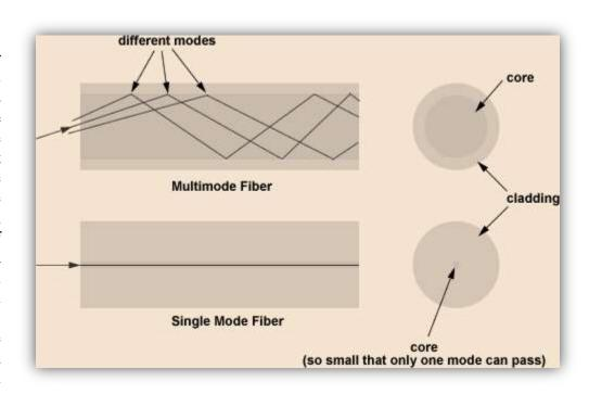
conditions that shape how light waves travel through the fiber, like the walls of a tunnel affect how sounds echo inside.
