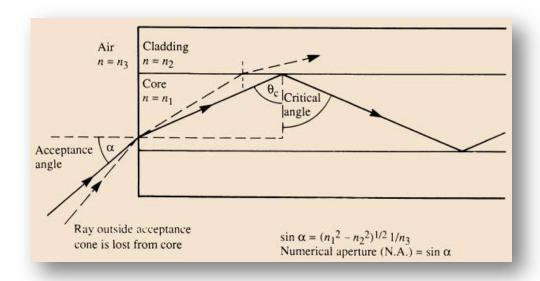
Acceptance angle is measured in air (refractive index  $\approx$  1) outside the fiber. The acceptance angle normally is measured as **Numerical Aperture** (**NA**), which for light entering a fiber from air is approximately
