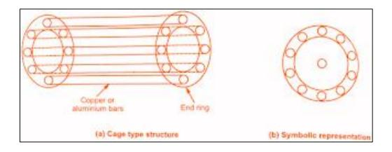
As the bars are permanently shorted to each other, the resistance of the entire rotor is very very small. The air gap between stator and rotor is kept uniform and as small as possible. The main feature of this rotor is that it automatically adjusts itself for the same the number of poles as that of the stator winding. The schematic diagram of two-pole **single phase induction motor** is shown in the below figure:
