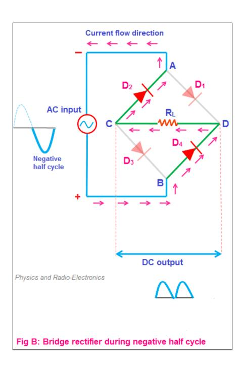
From the above two figures (A and B), we can observe that the direction of current flow across load resistor  $R_L$  is same during the positive half cycle and negative half cycle. Therefore, the polarity of the output DC signal is same for both positive and negative half cycles. The output DC signal polarity may be either completely positive or negative. In our case, it is completely positive. If the direction of diodes is reversed then we get a complete negative DC voltage.
