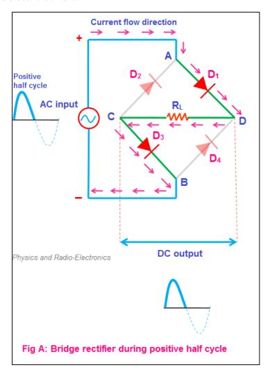
During the positive half cycle, the terminal A becomes positive while the terminal B becomes negative. This causes the diodes  $D_1$  and  $D_3$  forward biased and at the same time, it causes the diodes  $D_2$  and  $D_4$  reverse biased.
