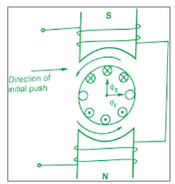
Now Fleming's left hand rule can be used to find the direction of the force experienced by the rotor conductors. It can be seen that when  $\Phi s$  acts in upward direction and increasing positively, the conductors on left experience force from left to right while conductors on right
