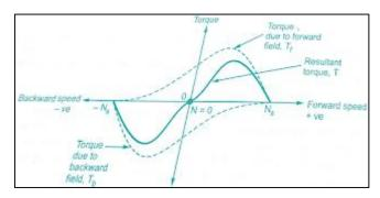
But in practice, it is not possible to give initial torque to rotor externally hence some modifications are done in the **construction of single phase induction motors** to make them self starting. Another theory which can also be used to explain **why single phase induction motor is not self starting** is cross-field theory.
