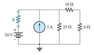
[10] Obtain the Thevenin's equivalent circuit for the following circuits,
