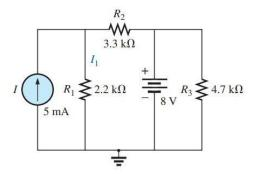
[9] Obtain Thevenin equivalent circuit for the network external to the resistor R for the givennetwork.
