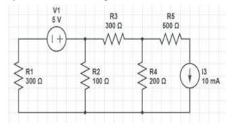
[8] Use the superposition theorem to find current through R1 for the given network
