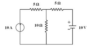
[12] For the following circuit, find the current I using the Norton's theorem.
