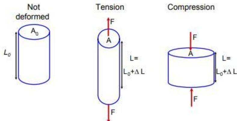
$\Delta L$  can be measured as a function of the applied force; area  $A_0$  changes in response
